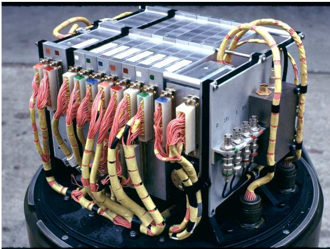
Figure 7: The main electronics assembly consisting of 8 vertical cards.
