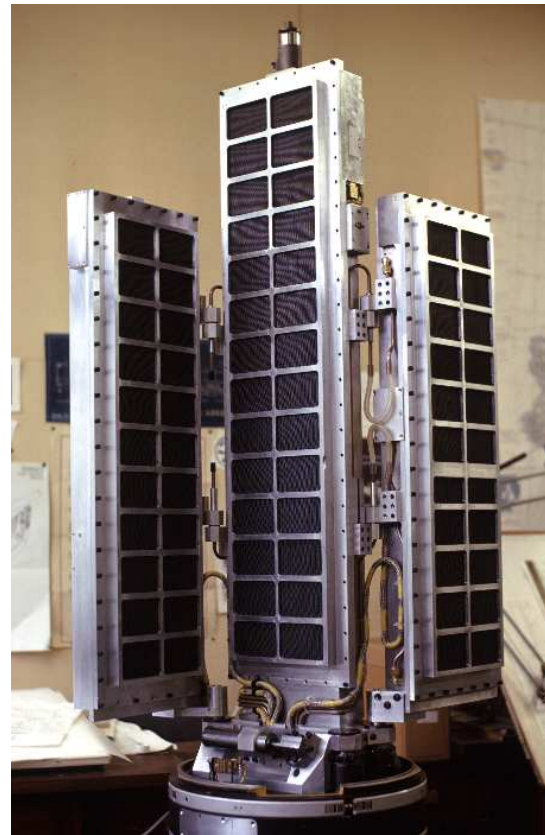
Figure 3: Experiment - partially deployed panels.
