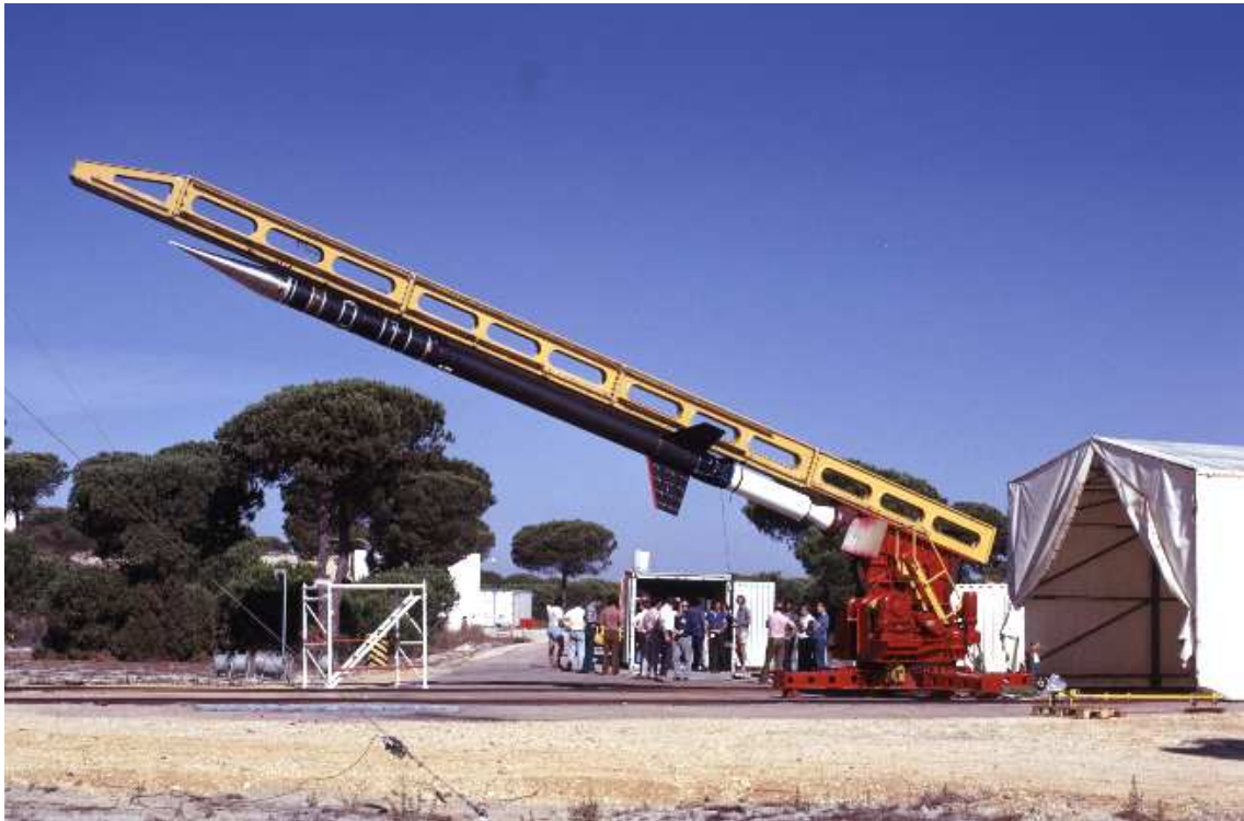
Figure 16: Launcher rail in semi-lowered position.
